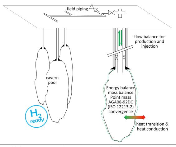
Calculation model of CavBase GasStorage for a single cavern as well as for a cavern pool operated in parallel.
