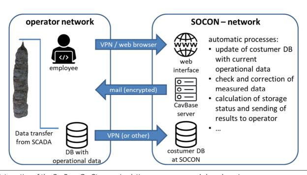
Integration of the CavBase GasStorage simulation program as a web-based service
